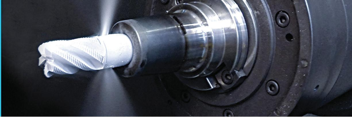
In the past, cryogenic machining was inefficient and ineffective, forcing many manufacturing facilities to stick with traditional coolants. The main problem with first generation cryogenic systems was that they utilized an external process, which allowed most of the cryogen to evaporate before reaching the cutting surface, ultimately reducing its cooling capacity.
