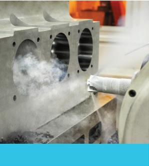
Conventional “wet” machining solutions negatively impact our environment in their production, use, and disposal of often-toxic cooling fluids. 5ME cryo is a “dry” solution. When LN2 evaporates back into the atmosphere, it dissipates to – an inert, non-greenhouse gas.
